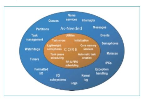
The **MQX™ RTOS** offers leading-edge technology for embedded designs based on the Atmel AT91 family processors.
